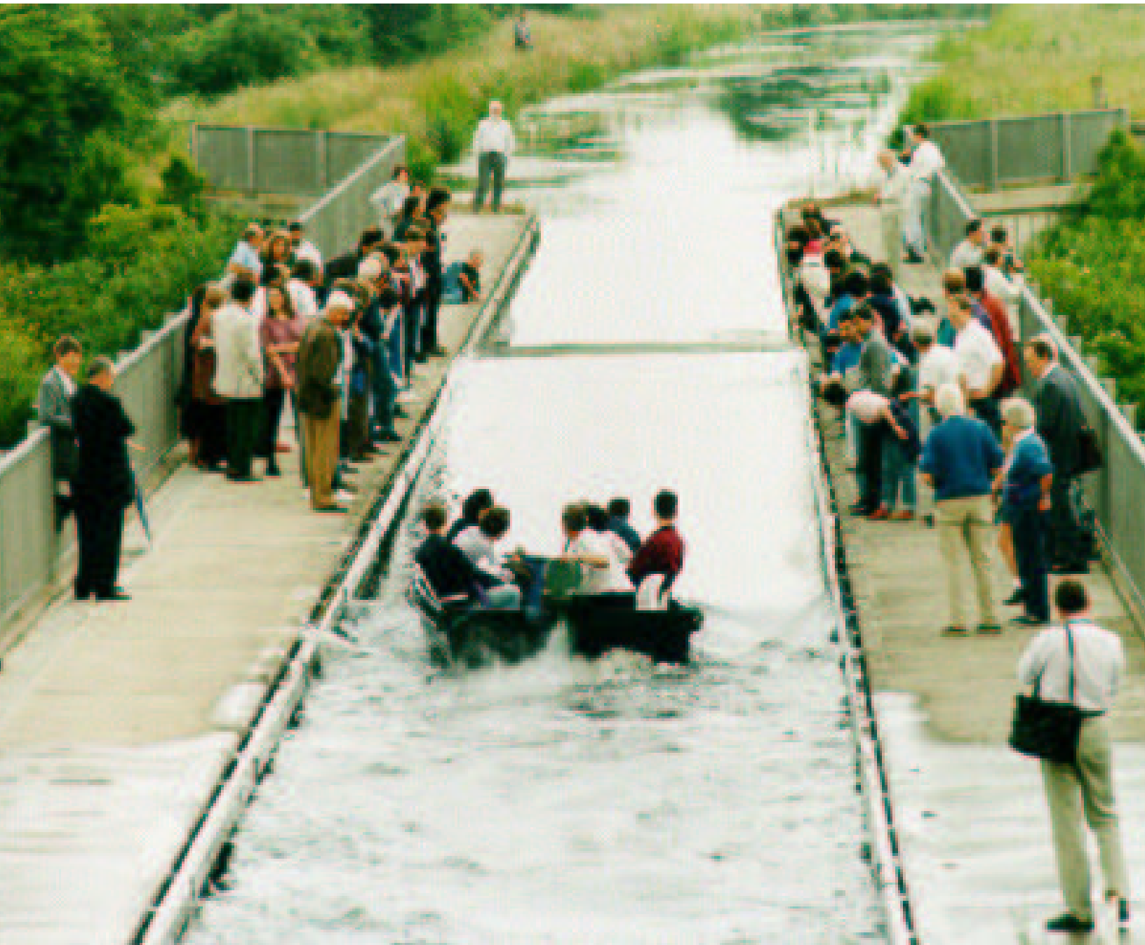
Soliton on the Scott Russell Aqueduct on the Union Canal near Heriot-Watt University, 12 July 1995 (Photo from Dugald Duncan, Heriot-Watt University, Edinburgh).
