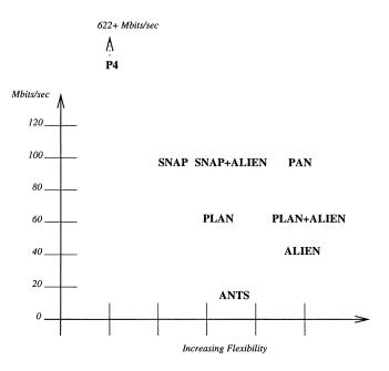
Fig. 10. Flexibility versus measured performance tradeoffs.
