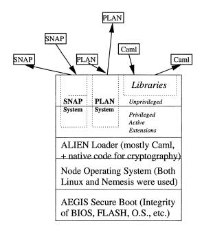
Fig. 9. SwitchWare system architecture.
