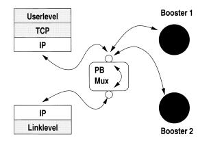
Fig. 5. Multiplexing of boosters in the 4.4 BSDlite IP stack.
