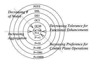
Fig. 11. Computation versus network performance tradeoffs.
