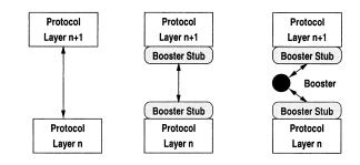
Fig. 4. Inserting a booster into a protocol stack.
