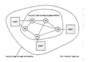
Fig. 1. Typical packet switching network.
