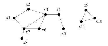
This network has 11 switches and 12 wires. It doesn't exactly look like the Internet, but it might represent a typical architecture of a single corporate network. The first strange
