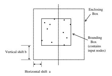
Fig. 2. The enclosing box contains the bounding box and is twice as large, but is shifted by random amounts in the x and y directions.
