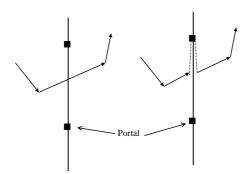
Fig. 4. Every crossing is moved to the nearest portal by adding a "detour."
