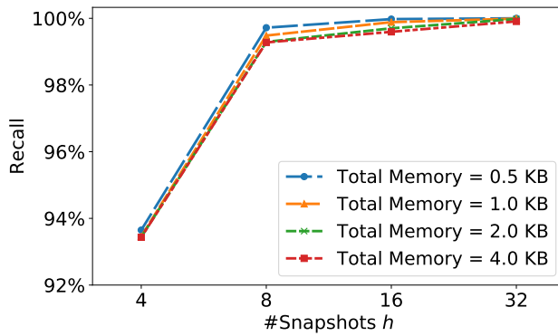
Figure 5.6: Recall vs. number of snapshots. Using 8 snapshots gives sufficiently high Recall.
