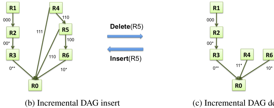
Figure 3.2: Constructing the rule dependency graph (edges annotated with reachable packets)
