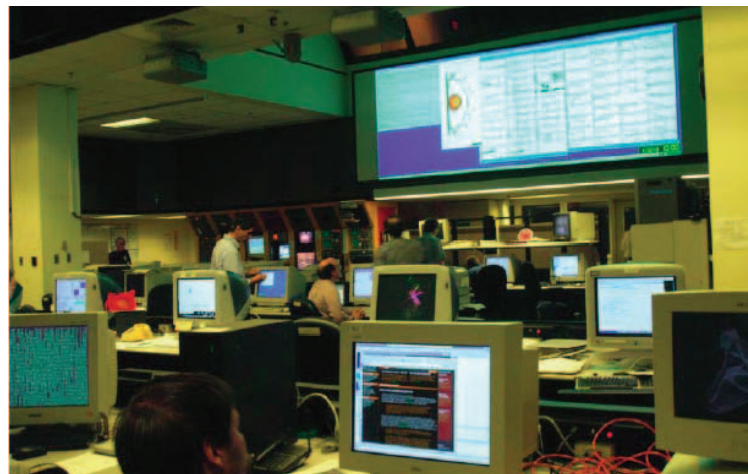
13 Shared display using multicursor X and application sharing in the control room of Princeton Plasma Physics Lab.
