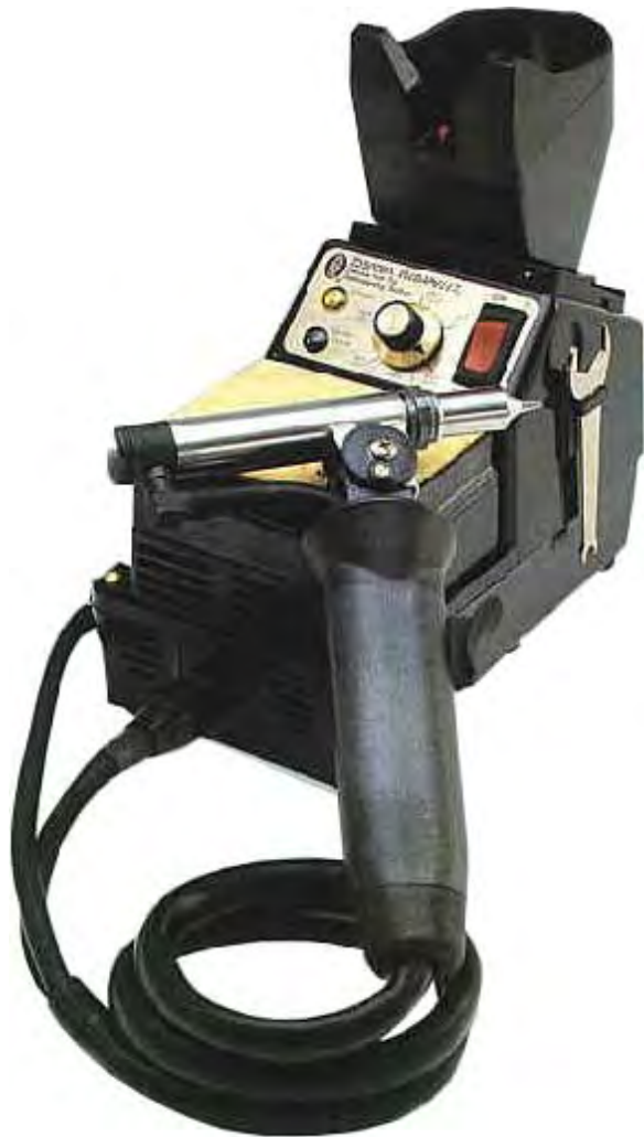
Figure 18: Desoldering tool uses heat to melt the solder and a vacuum pump to suck it out of the joint. Can be used to remove Z80 processor chip from AVC Advantage motherboard.
