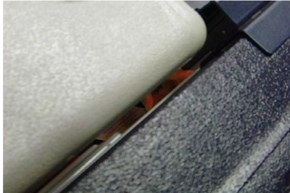
Figure 26: Peeking through the slot at the position of the voter's finger. Here, the pollworker can see that the voter is voting for a candidate at the left side of the full-face ballot. This shows more clearly in the video that accompanies this report.
