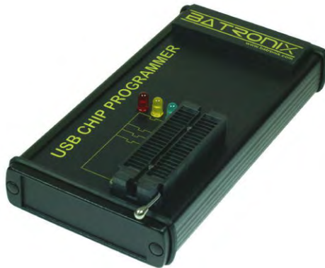
Figure 8: ROM reader/programmer; cost $150; approx. 3 inches by 2 inches
