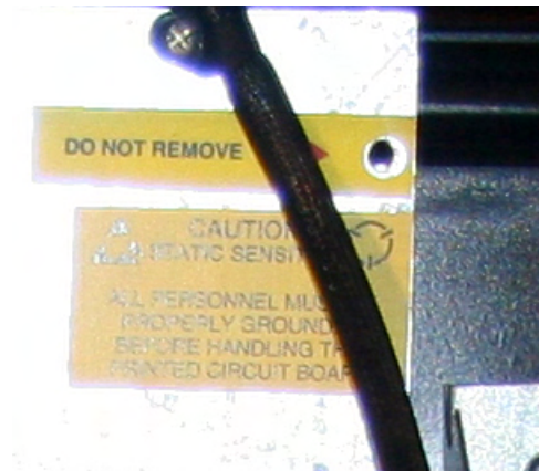
Figure 14: Close-up from Figure 5. The hole labeled DO NOT REMOVE contains no seal.
