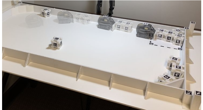
Fig. 10. Emergent behaviors. An Anki Vector robot executes a policy learned in simulation. It first pushes objects towards the wall, then uses the wall as a guide to simultaneously push several objects until they are all in the receptacle.
