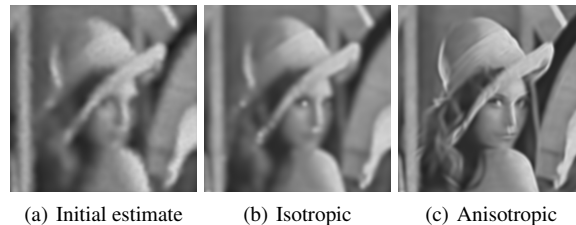
Figure 4: Starting from the initial estimate, our optimization can compute either isotropic or anisotropic approximations. Due to the significant qualitative improvement, we always use anisotropic Gaussians for our surfaces.
