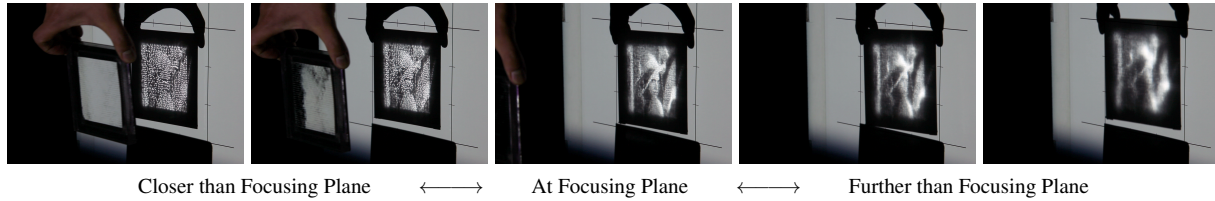
Figure 13: Positioning the sample at different distances to the projection plane shows the effective depth of field of the caustic.
