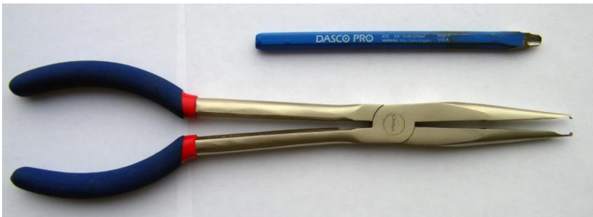
Fig. 15. (top) chisel ground to radius of cup; (bottom) pliers ground to grip and remove cap from base.
