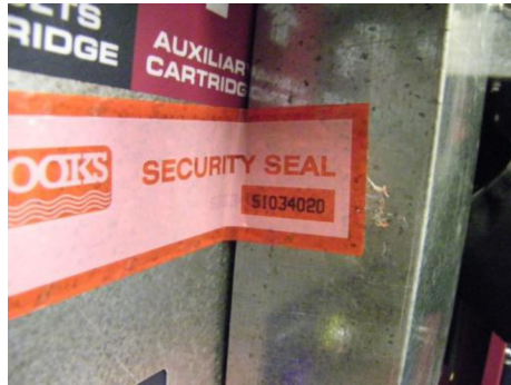
Fig. 22. Sticky adhesive tape seal.
