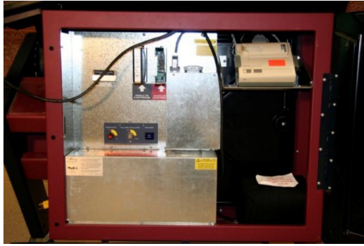
Fig. 2. Rear of AVC Advantage cabinet with door open (hinge at right).
