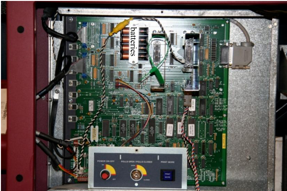
Fig. 3. Circuit-board cover removed from motherboard enclosure. Bottom center, panel for on/off knob. Top center (just to the right of “batteries”), a green strap seal remaining after the circuit-board cover has been moved past it (see discussion of seal regime #1). Slightly to the lower right of center, 1 configuration ROM and 3 program ROMs with white labels. At top left and top center of enclosure, one can see two of the 10 threaded holes for the screws that hold the circuit-board cover in place.
