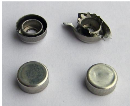
Fig. 16. Small cup “seal”. Top left, base; bottom left, cap; top right, base after removal; bottom right, cap after removal.
